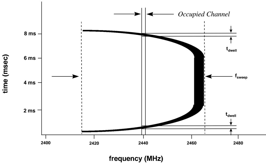
**Figure I-2 Spectrographic Plot of Microwave Oven Interference**
